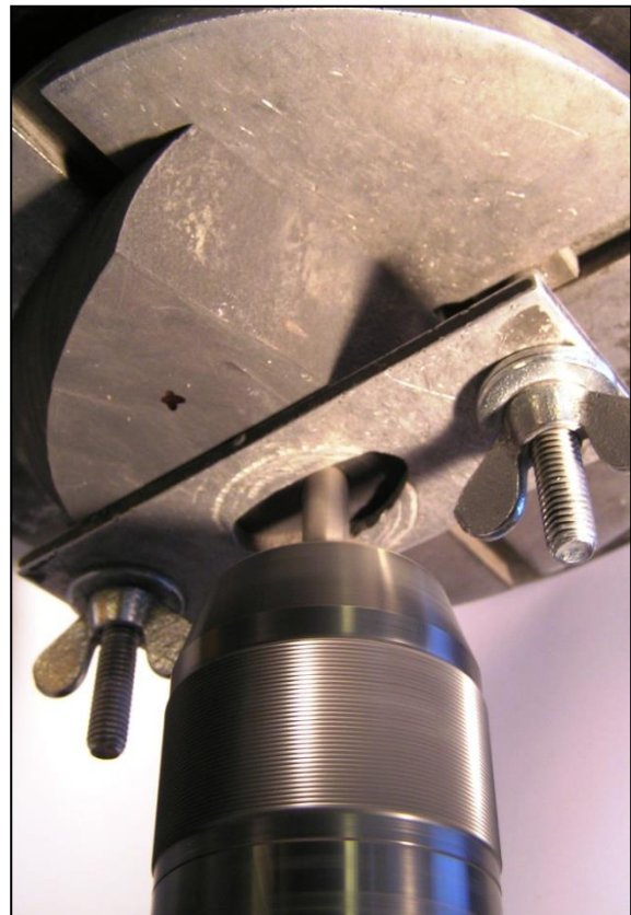
Close up of drill and Sievers' J piece.
