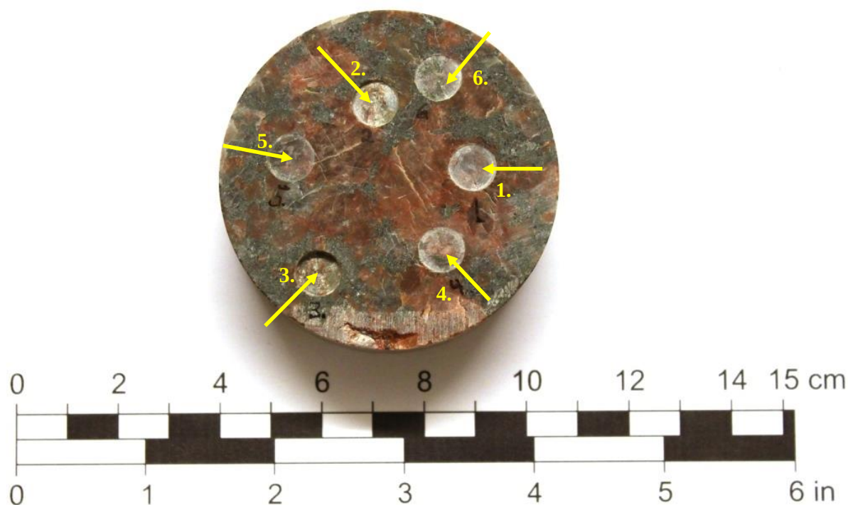
Photo of the Sievers' J (SJ) specimen subsequent to completed testing. Yellow arrows and figures indicate the position of the drillings.
