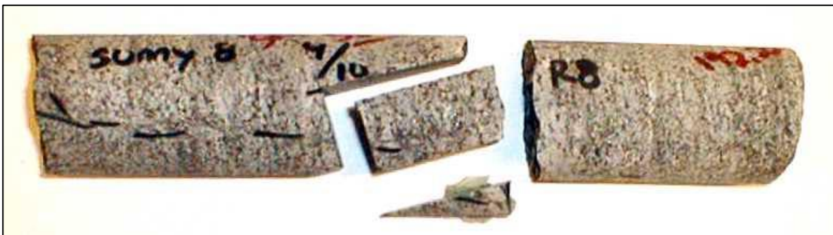
A section of a rock core sample showing the orientation of the pre-cut Sievers' J piece in relation to the core axis and foliation.
