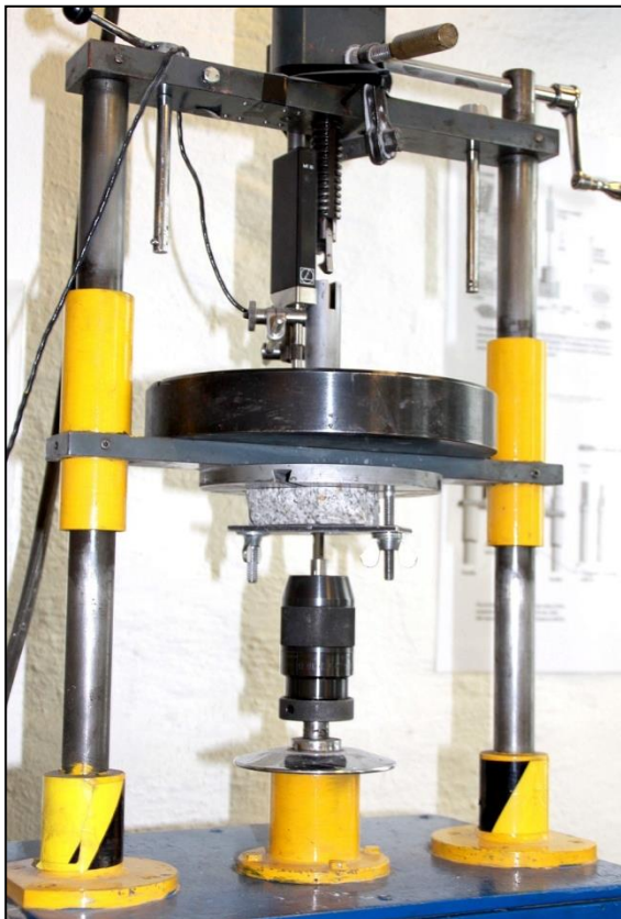
Sievers' J-Value test equipment.
