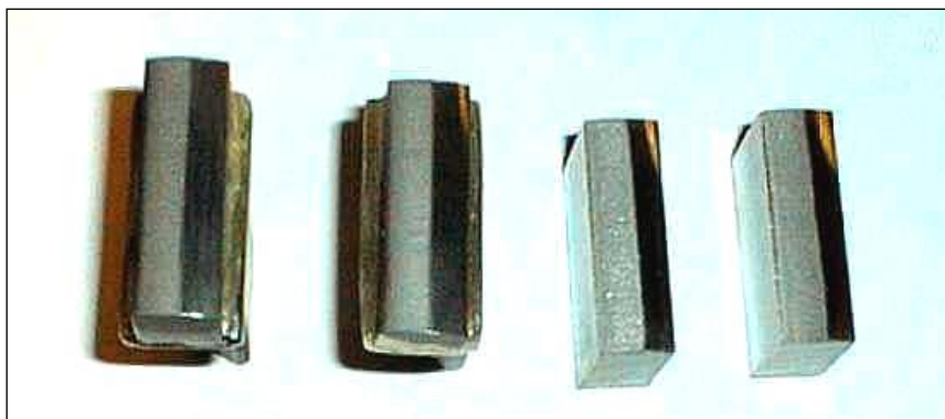
AV (left) and AVS (right) test pieces subsequent to testing. For scale, the right-hand test piece is 30 mm long.
