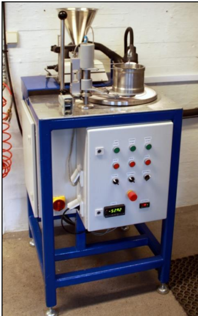
Test equipment used to determine Abrasion Value (AV) and Abrasion Value Cutter Steel (AVS).
