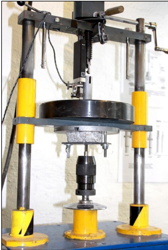
Sievers' J-Value test equipment.
