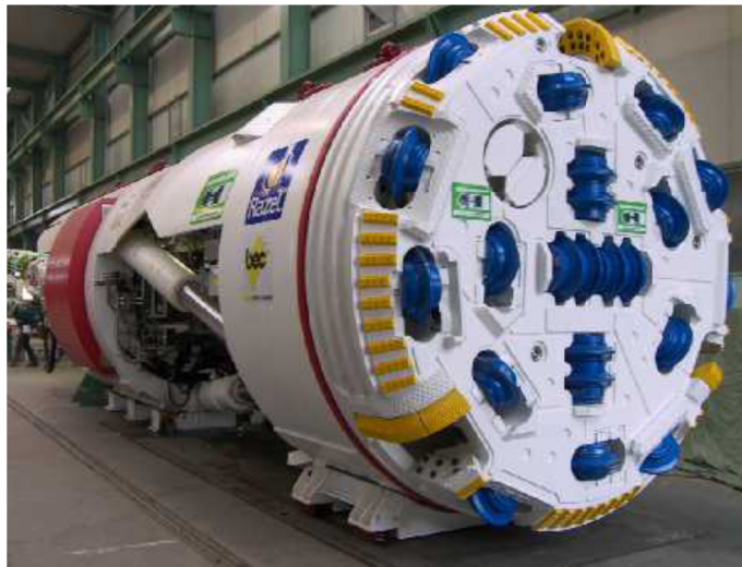
Figure 5 Gripper TBM with a boring diameter of 3.5 m [21]
